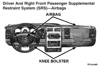
This vehicle has airbags for both the driver and right front passenger as a supplement to the seat belt restraint systems. The driver's front airbag is mounted in the steering wheel. The passenger front airbag is mounted in
